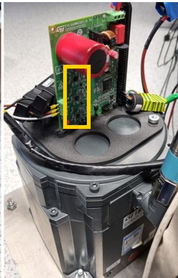
GaN Inverter with 3x STDRIVEG611
