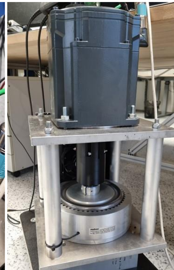
Motor brake joint with 3D printed clutch
